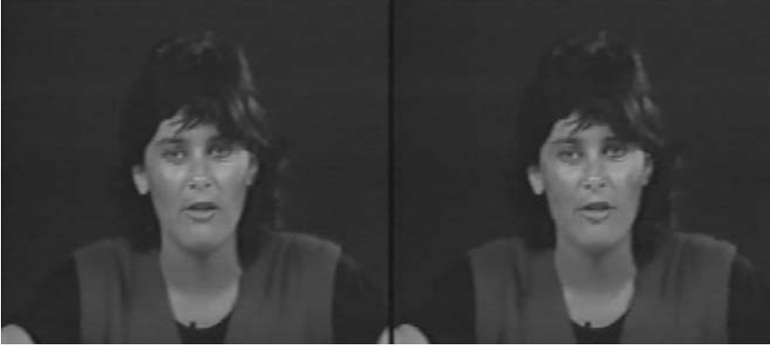
Figure 6. Original (left) and reconstructed (right) frame from the sequence Miss America, using a global codebook with 2 \times 2 \times 4 blocks. The compression here is 14:1.
