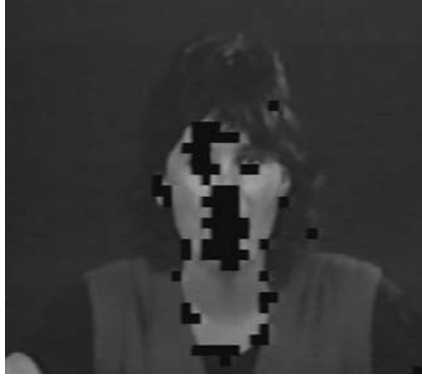
Figure 5. Reconstructed frame based on vectors found in localized codebooks, as shown in the block diagram of Figure 2. Black areas were not encoded properly in this stage and are searched for best match in adjacent codebooks in the second stage (Figure 3).
