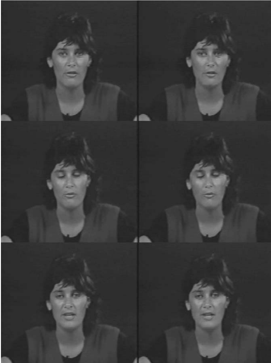
Figure 9. Comparison of the Global approach (left, 62:1) to the localized version (right, 100:1).
