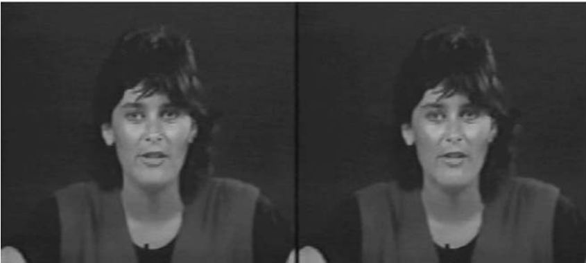
Figure 8. Original (left) and reconstructed (right) frame from the sequence Miss America, using localized codebooks with 4 \times 4 \times 4 blocks. The compression is 100:1.
